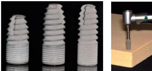
Fig. 1 (left): Implant dimensions used in this study: (left) Implant dimension 4.8 × 10 mm; (center) implant dimension 4.8 × 12.5 mm; (right) Implant dimensions 4.1 × 12.5 mm; Fig. 2 (right): The implants were inserted into laminated polyurethane foam using a surgical motor capable of recording the actual torque applied over time.
